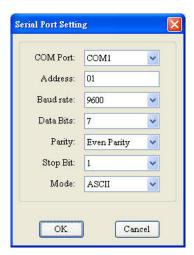
(3) Set up the communication parameters in the PC and DVP-SV, e.g. the communication port, address, baud rate and communication format.
