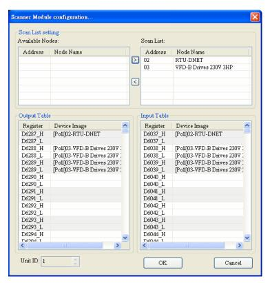
(3) Confirm all the settings and click on "OK". Next, download the configuration to DVPDNET-SL. If DVP-SV is in RUN mode while you are downloading the configuration, a "Warning" dialog box will appear.
