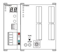
The index of DVPDNET-SL is its number. The first DVPDNET-SL on the left hand side of DVP-SV is No. 1, the following DVPDNET-SL modules are No.2, No.3, No.4 and so on.
