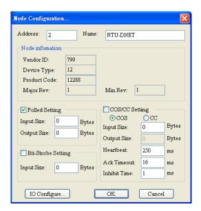
(8) Click on "IO Configure..." button in "Node Configuration" dialog box, and you will then see "RTU Configuration" page.
