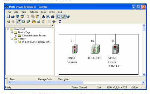
(7) Double click on RTU-DNET (node 02), and the "Node Configuration..." dialog box will appear.
