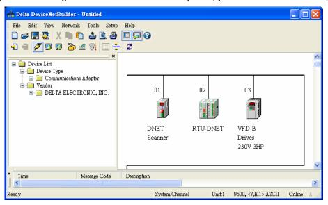
(15) Double click on VFD-B Drives (node 03), and the "Node Configuration..." dialog box will appear.
