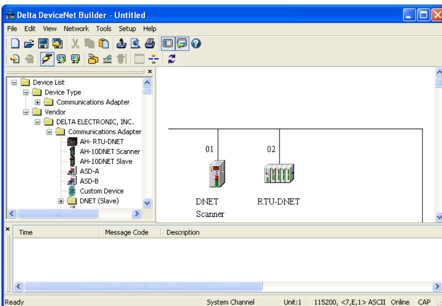
7. Double click on RTU-DNET icon (node 2), and the “Node Configuration” box shows up.
