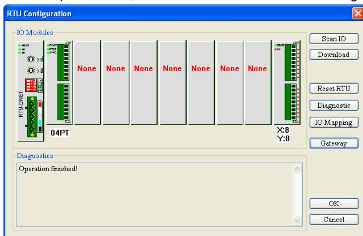
14. Double click "RTU-DNET" icon and then "RTU Setup" page appears. You can see 4.2.2 for explanation of the parameters in the following page.
