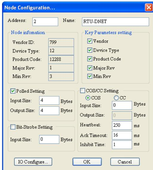
8. Click on “IO Configure...” button in “Node Configuration” dialog box, and you will then see “RTU Configuration” page.
