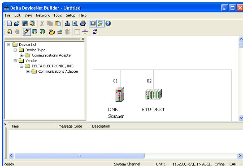
(6) Choose “RTU-DNET” icon, then press the right button of the mouse, finally select “Parameter Edit...” in the following menu to enter “Parameters Edit...” page.
