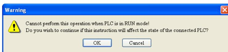
4. Click on “OK” to continue the download. Make sure DVP-SV is in RUN mode. Now, you can see the MS LED and NS LED on RTU-DNET and DVP-SV become green. And LED nixie tube of DVPDNET shows “01”.
