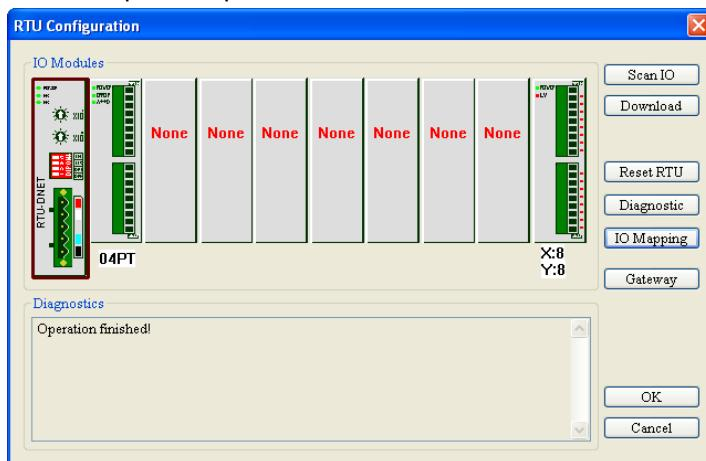
16. Double click “04PT” and then “Special Module Configuration” dialog box displays. For the parameter explanation, see 4.2.3.
