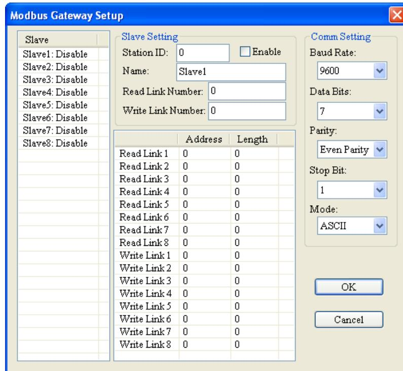
12. Set up the parameters in the above dialog box and see 4.2.4 for explanation of the parameters.
