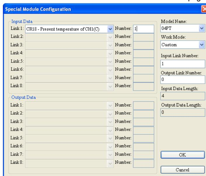
18. Click on “OK” in the above “Special Module Configuration” page after confirming the configuration data set up. Next, click “Download” in the “RTU-DNET configuration” page to download the configuration data to RTU-DNET. After download is completed, click on “OK”.
