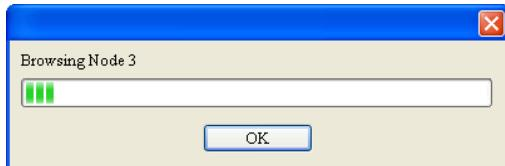
(5) If the bar on the dialog box does not progress, it means the connection between the PC and DVP-SV is abnormal, or there are other programs also using the COM port on the PC. After the scan is completed, the dialog box will tell you that the scan is completed, and the icons and device names of all the nodes scanned on the network will be shown on the screen. See the figure below, in which the node address of DVPDNET-SL is 01.
