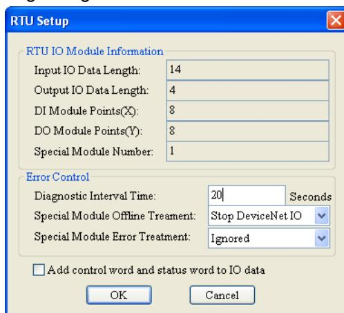
Explanation of RTU setup parameters:
