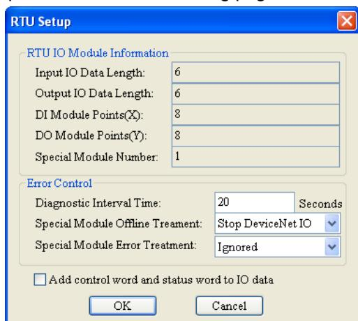
15. After setup is completed, click on “OK” to return to “RTU configuration” page.
