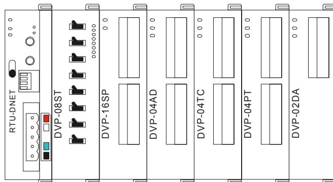
■ DVP Slim DI/DO extension units connectable to RTU-DNET
