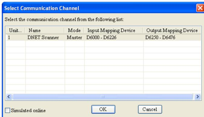
(4) Click on “OK” button and then DeviceNetBuilder software starts scanning the network.
