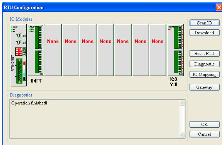
11. Click on “Gateway” button to enter the “MODBUS Gateway Setup” dialog box.
