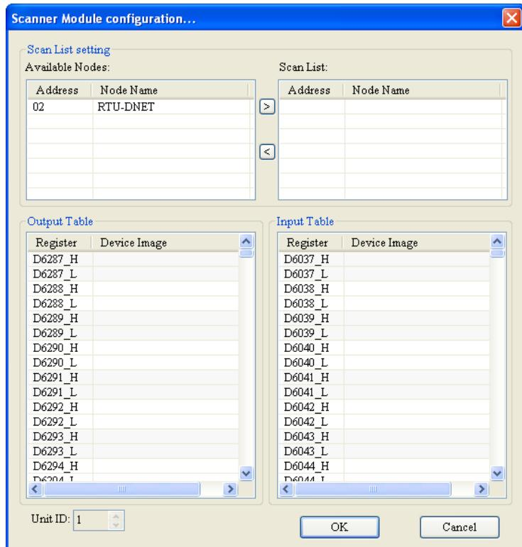
2. Move the slave devices on DeviceNet in the “Available Nodes” list on the left side to the “Scan List” on the right side. Select a node and click on . Follow the steps to move all the nodes to the scan list.
