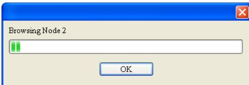
6. If the bar on the dialog box does not progress, it means the connection between the PC and DVP-SV is abnormal, or there are other programs also using the COM port on the PC. After the scan is completed, the dialog box will tell you that the scan is completed, and the icons and device names of all the nodes scanned on the network will be shown on the screen. See the figure below, in which the node address of DVPDNET-SL is 01.
