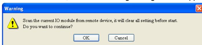
10. Click on “OK”. DeviceNet Builder will then detect the special module connected to RTU-DNET and the number of points in the Slim DI/DO extension unit and display the information on “RTU Configuration” page.
