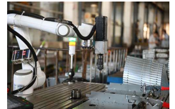
Drilling metal sheets
