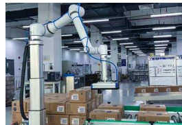
Palletizing with lifting column and custom-made gripper extender
