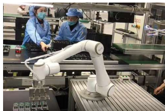
Pick & place of PCB boards
